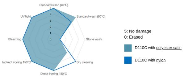
These performances are for guidance only. Results are obtained with adapted receiving material and optimum print conditions. (Ricoh test method)
